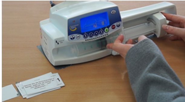
Fig. 8 Screenshot of the Video Analysis During the Skills Test. On the left, the current task (i.e., task number 1: switch on syringe pump, insert the syringe, and choose “—no medication—”) is displayed on a card. The location of the syringe pump was marked with tape on the table to ensure that the video captured all relevant actions
